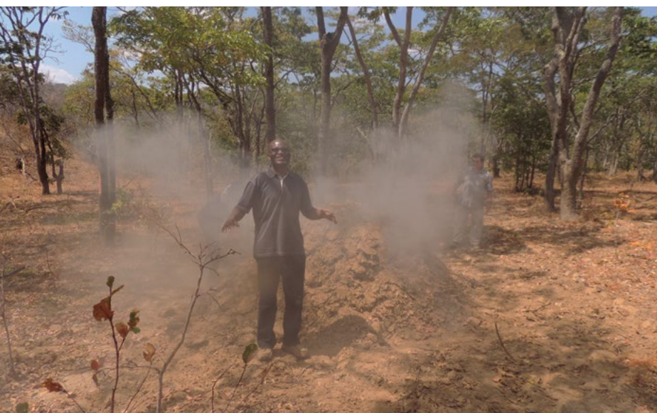
Drs. Zulu and Skole view an earth charcoal kiln in Perekezi Forest Reserve, northern Malawi. Traditional earth kilns are wasteful, requiring 8-10 tons of wood to produce a ton of charcoal.
